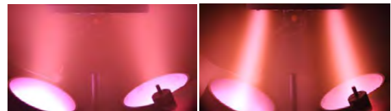
Fig. 3: View of the sputter deposition chamber, with the substrate holder at the top. The effect of an additional magnetic field (right side) on the plasma confinement is clearly visible.
