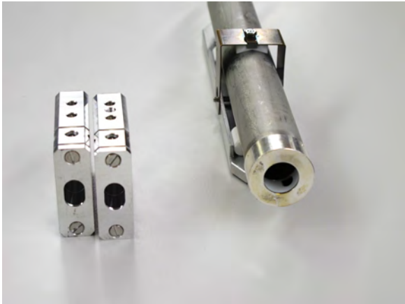
Fig. 1: New Faraday Cups (left) compared to the previous cups (right).
