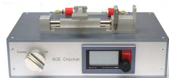
Fig. 2: Tube cracker system for the automated graphitization line AGE.
