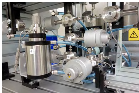
Fig. 2: Pneumatic valves for automated gas extraction.
